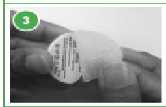
Peel off the transmitter adhesive to remove the adhesive pad from the transmitter.
